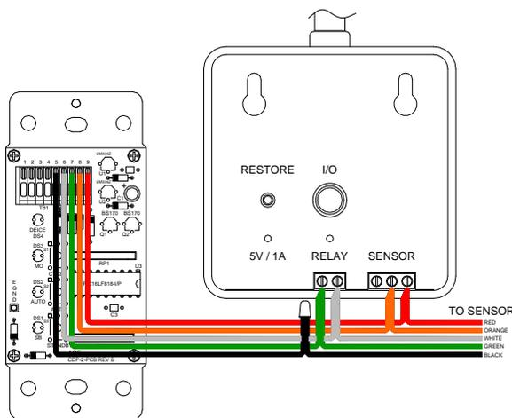
Though CDP-2 control will be temporarily lost this is a valid and safe mode of operation if the functions described are needed. Though not shown, the interconnect cable used from sensor to WeMo Maker should always be shielded, stranded, tinned copper leads (CS-50 style) with the shield drain wire terminated to earth ground on one end only. The same is true if extending the WeMo Maker to a CDP-2.
